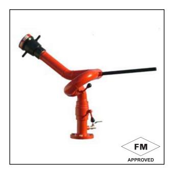
The vertical and horizontal rotation is through corrosion resistant swiveling joints with double row of stainless steel ball bearing. Both vertical and horizontal movements are controlled by handle and twist lock.
